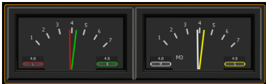
Example: PPM display in Dual L/R mode left beside Dual M/S mode with horizontal orientation of TM3
